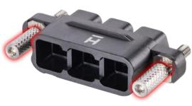
Contacts on the Kona range are all individually shrouded, with a recessed design. This helps prevent accidental touch of contacts by locating the contact end below the housing face. The contacts are also better protected against incidental damage from physical knocks or mis-mating.
